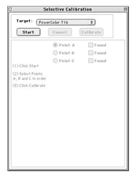
Figure 5–2 Selective Calibration window
